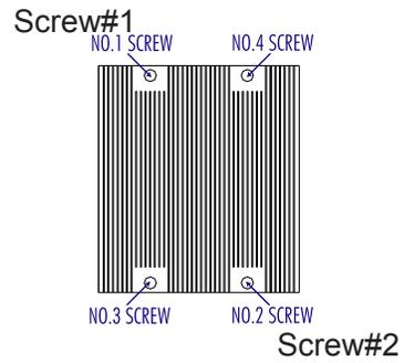
2. Hold the heatsink as shown in the picture on the right and gently wriggle the heatsink to loosen it from the CPU. (Do not use excessive force when wriggling the heatsink.)
