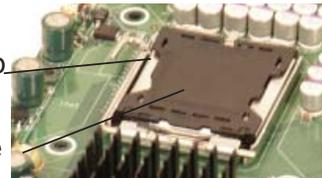
1. Press the socket clip to release the load plate, which covers the CPU socket, from its locking position.
