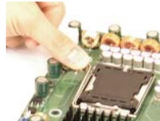
2. Gently lift the socket clip to open the load plate.
