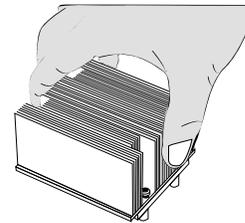
4. Clean the surface of the CPU and the heatsink to get rid of the old thermal grease. Reapply the proper amount of thermal grease on the surface before you re-install the CPU and the heatsink.
