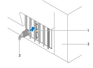
Figure 4-3. Connecting the Cable From the External Enclosure
