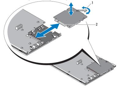
Figure 4-14. Removing and Installing the Storage Controller Card
