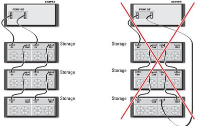
**Redundant Path Support Configuration With Three Enclosures** Figure 4-13.
