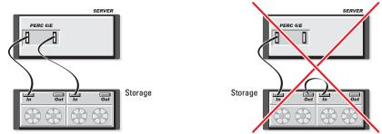
Figure 4-12 displays Redundant path Storage Configuration with two enclosures.
