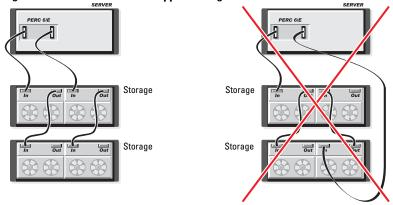
Figure 4-13 displays Redundant path Storage Configuration with three enclosures
