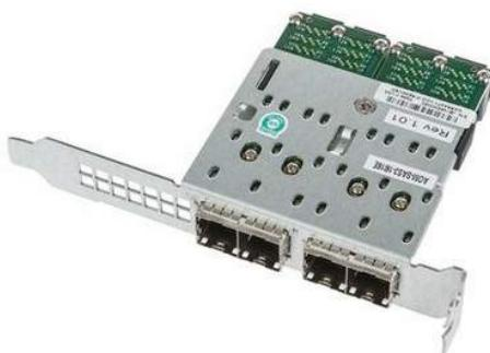
**Figure C-17.** Mini-SAS HD Internal to External Adapter
