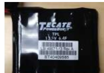
#2: CVPM02 (CacheVault Power Module)
