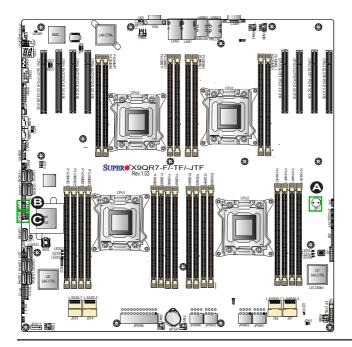
A. Internal Speaker (Buzzer) B. T-SGPIO1 C. T-SGPIO2 D. T-SGPIO3
