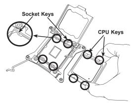
Once they are aligned, carefully lower the CPU straight down into the socket.
