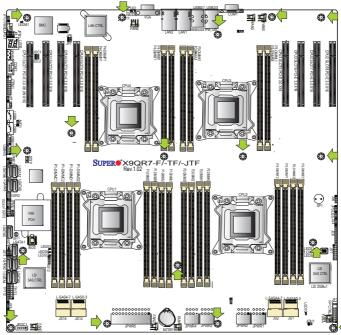
**Warning:** 1) To avoid damaging the motherboard and its components, please do not use a force greater than 8 lb/inch on each mounting screw during motherboard installation. 2) Some components are very close to the mounting holes. Please take precautionary measures to prevent damage to these components when installing the motherboard to the chassis.
