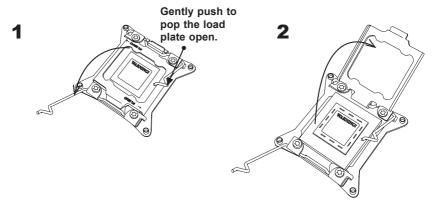
1. Use your index fingers to loosen the lever and open the load plate.
