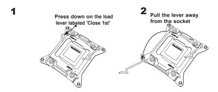
With the lever labeled 'Close 1st' fully retracted, gently push down on the lever marked 'Open 1st' to open the load plate. Lift the load plate to open it completely.
