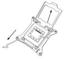
Use your thumb and index finger to hold the CPU on its edges. Align the CPU keys, which are semi-circle cutouts, against the socket keys.
